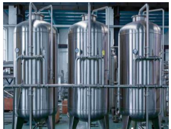
Pic.1 Water filter system
